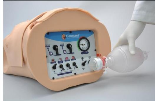
3. Slowly begin pumping to pressurize. Monitor the "Air Pressure" dial closely and **STOP** pumping when the Air Pressure dial reaches the **3 psi mark**.
