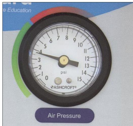
Do not exceed the recommended pressure marked green. Filling the system beyond its capacity will stress the internal mechanics and cause damage the simulator.
