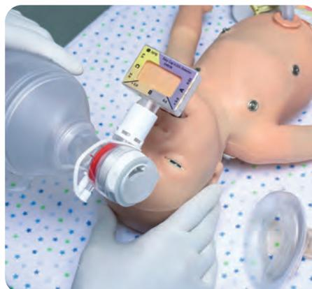
Detect CO<sub>2</sub> exhalation using real devices
